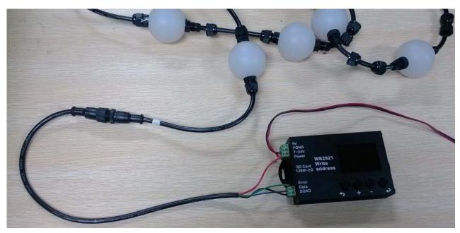
Disconnect from power prior to making any connections. Connect the DMXSphere strand of spheres to the address writer as shown above. It will require an external power supply between 12 and 24vDC to power the DMXSpheres. We suggest using the same power supply that will supply the DMXSpheres with 15vDC.
