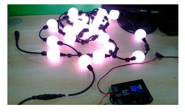
Once the DMXSphere is programmed, the strand will go all white. Turn off or disconnect the power supply. The strand is now set and may be disconnected and connected to power and DMX using the proper cables. Repeat the steps above to program the start address of another strand.
