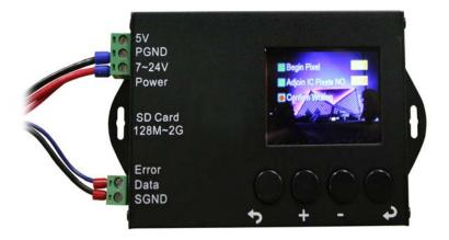
With the red selector in the first box, Begin Pixel, set this number to be the number of the first sphere in the strand. Leave the Adjoin IC Pixels NO. set to 0. Once you have set the number of the first sphere also known as a pixel in the strand, use the -/+ buttons to move to the Confirm Writing box. Press enter button.
