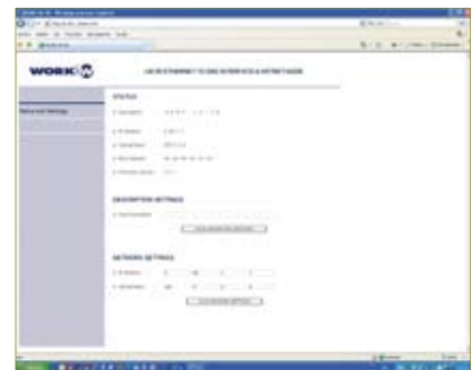
Integrated WEB SERVER for LM-3E and LM-3R configuration. It is possible to edit IP address and unit description.
