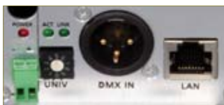
LM-3E and LM-3R front panels with LAN connection, group selector and LED for DMX and Ethernet signal.
