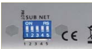
LM-3R rear panel with DIP switch block for protocol selection ( WorkNet or standard ArtNet and Subnet mask).
