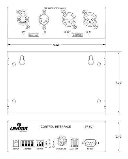
The Leviton-NSI I/F 501 Control Interface is your simple solution for dimmer and control systems compatibility. Increased flexibility of control system design is achieved with the multiple signal ports and protocols available with the I/F 501. The I/F 501 may be configured to combine and convert analog, analog multi-plex and digital control signals.
