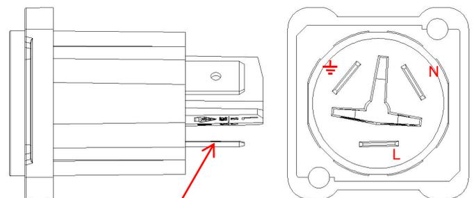
Soldering / plugging 6.3x0.8 terminals
