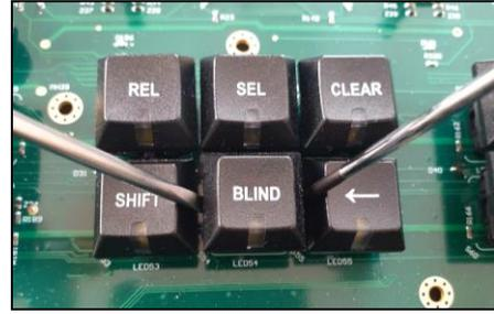
Next, de-solder the LED connections if an LED is fitted to the switch. If no LED is present, skip this part. The LED connections are the two at the bottom of the switch which are close together. Once fully de-soldered, remove the LED and remember its orientation. This is important for when it is re-fitted.
