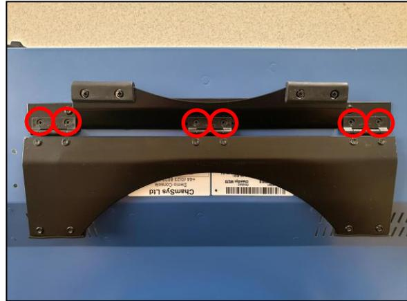
The front 2x feet can be removed by simply unscrewing the 2x M3x6 black screws in each foot using a PZ1 screwdriver.
