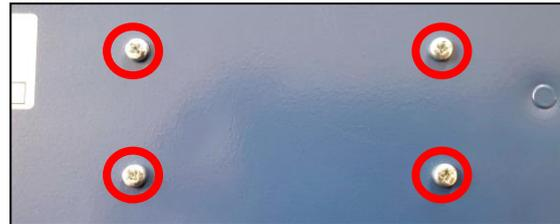
The power supply will then be loose to be removed and replaced, if required.
