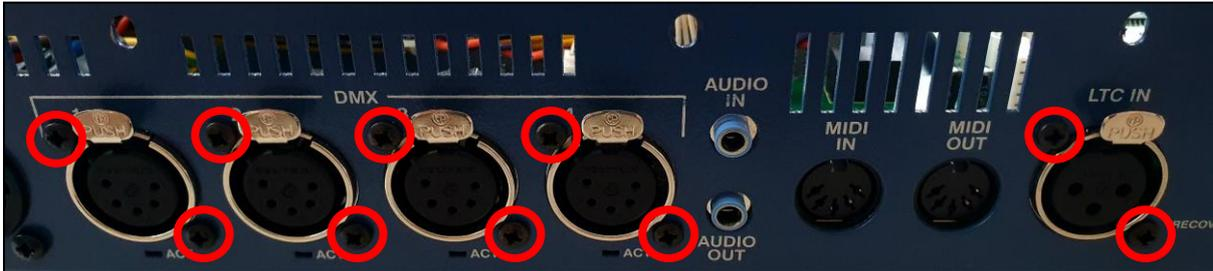
2. Disconnect the 2x cables as highlighted red in the image below. Both can simply be pulled off with a little force.
