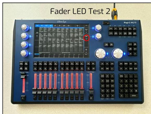
You can also run through a full production test using the PROD TEST soft key on screen in board test mode, but some specific testing equipment is required for testing some other functions on the console, such as the DMX, Network and Midi ports.
