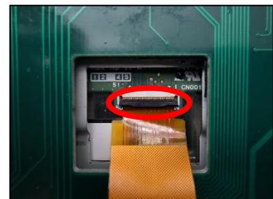
If the display doesn't work after re-fitting this cable, try re-seating it again. This can be difficult to seat correctly.
