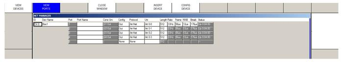
The rate, frame, MAB and Break timing can be set for each interface – the timings affect all ports on the interface.
