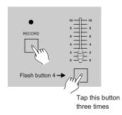
Tap the Flash button 4 three times while holding down the Record button, the Segment Display reads "OUT" indicating the controller is ready to send a file.
