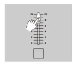
4. Move the desired Ch. slider 13-24 (25-48) to its maximum position to trigger the program, and the program will fade in depending upon current fade time.
