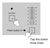
Tap the Flash button 2 three times while holding down the Record button, the Segment Display reads "CHO" indicating MIDI OUT channel setup is available.
