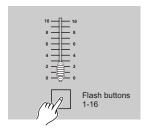
Tap the Flash button numbered from 1-16 to assign MIDI OUT channel 1-16, the relevant channel LED lights indicating MIDI OUT channel is set.
