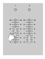
3. Create a desired scene using Channel Sliders 1-24 (1-48). At 0% or DMX 0, these sliders should be at 0 position, and at 100% or DMX 255, these sliders should be at 10 position.
