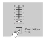
Tap the Flash button numbered from 1-16 to assign MIDI IN channel 1-16, the relevant channel LED lights indicating MIDI IN channel is set.
