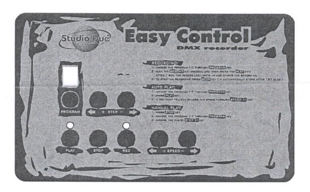
The Easy Control is a small DMX recorder that can solve many problems in small installations, when the price of a DMX controller is too high and therefore not acceptable.
