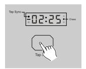
In Chase mode, repeatedly tapping the Tap Sync button establishes the chase speed. The last two taps determine the speed with a maximum of 5 minutes and the Tap Sync indication in the Segment Display lights. Tap Sync will override any previous setting of the Speed/Fade Time knob unless you adjust the Speed/Fade Time knob again.
