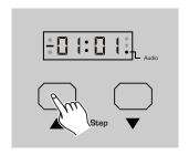
2. Tap the Step Up/Down button until the Segment Display shows "01" in the right two characters.
