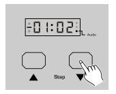
4. Tap the Step Up/Down button until the Segment Display shows "02" in the right two characters.
