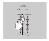
7. Move the Master Slider slowly up, the A LED fades in and the B LED fades out, the channel 1 fades down and the channel 2 fades up.
