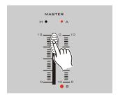
3. Move the Master Slider to top, the M LED lights at full intensity.
