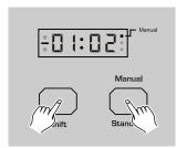
Keep pressing the Shift button, tap the Manual button until the Manual indication in the Segment Display lights indicating Manual is active.
