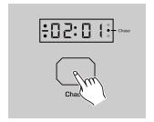
Tap the Chase button, the Chase indication in the Segment Display lights indicating Chase mode is active.
