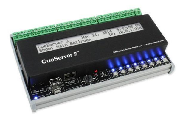
The CueServer 2 DIN is housed in an enclosure with replaceable side brackets suitable for DIN-Rail or surface mounting. It features a single LAN port, two DMX input ports and two DMX output ports. See the <u>CS-940 CueServer 2 DIN</u> section for more details for this model.
