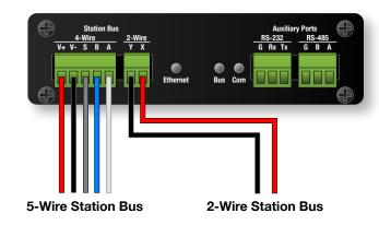
A maximum of fifty (50) 5-Wire stations can be connected to a single CueStation Hub. The maximum distance from the Hub to the farthest 5-Wire Station is 4000 feet (1220m).
