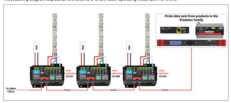
**Note:** when using CVC4s with any product within the Pixelator Family, set the P-Link port you have connected your CVC4s to output WS2812b with colour ordering RGB. This will convert your input DMX signal 1:1 into P-Link allowing you to mix and match CVC4 operating modes within the same String and patch them within your lighting control software.
