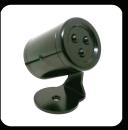
These IR emitters are installed into each scene where you want to control the Gantom Torch or other BlinkFX compatible devices. No DMX knowledge is required for setup using our free DMX Programmer app. Just connect your mobile device to the MiniEmitter and select the effect for each scene.
