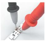
PUSH PROBES THROUGH PROTECTIVE SILICONE TO MAKE CONTACT
