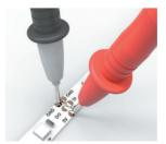
**PUSH PROBES** THROUGH **PROTECTIVE** SILICONE TO MAKE CONTACT
