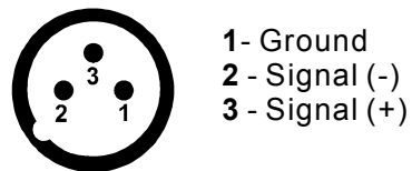
DMX-OUT XLR Connector - Socket:
