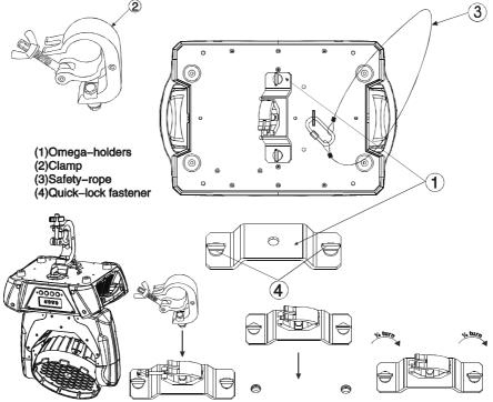
Screw one clamp each via a M12 screw and nut onto the Omega holders.
