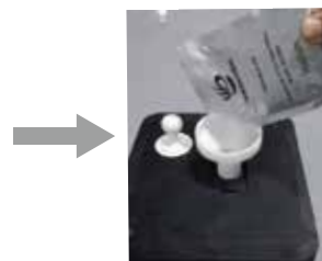
Filling the hopper
