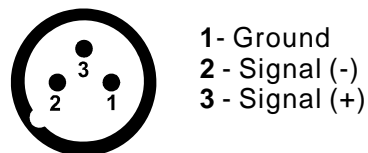
DMX-OUT XLR Connector - Socket:
