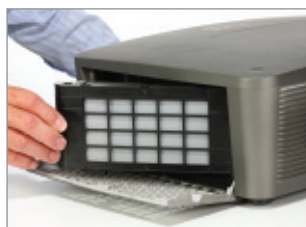
Replaceable air filter cartridge.
