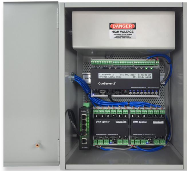
Example DE-1612 with (1) CS-940, (2) IT-SP8D splitters, Ethernet switch, and High Voltage Barrier installed
