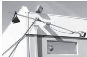
Speed rail pipe to wrap around corners.
