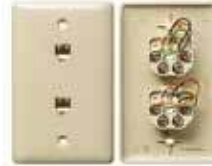
1-Gang Plate, Duplex RJ11 Jacks, 6-Position, 4-Conductor, Screw Terminations
