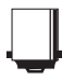
BA 15s DIN: 49720 IEC: 7004-11A ANSI: Single contact candelabra bayonet base C81.61-1990 sheet I-20-1
