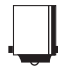
BA15d DIN: 49720 IEC: 7004-11A ANSI: Candelabra bayonet base double contact C81.61-1990 sheet I-20-1
